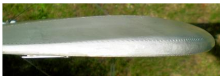
The author's Howard Pete has washout in only the last rib bay enough for a nearly constant chord wing. Washout in the Pete wingtip is formed by shaping the leading edge in the outer rib bay.
