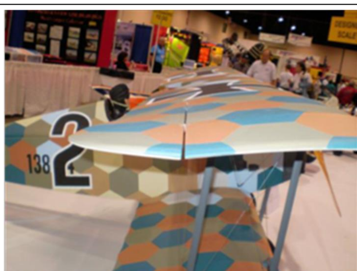
Martin Irvine's Aviatik D1 has washout confined to the ailerons. This common practice in WWI was a structural expedient that simplified assembly.
