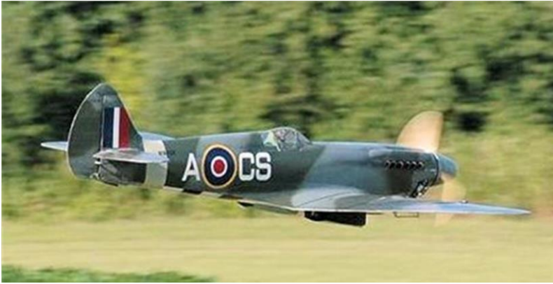
Despite its thin and pointed wingtips, Dave Szabo's Spitfire has excellent handling due, in part, to about 2 1/2 degrees of washout, slightly more than the full-sized Spit. low pass before a chandelle shown here.
