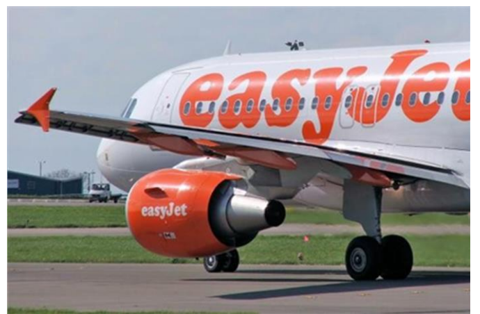
The thin wing of the Airbus A320 has lots of washout for safety.
