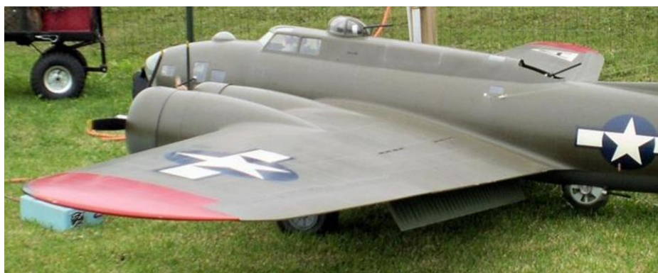
Washout provides good yaw control in Greg Hahn's B-17 in case of engine failure.
