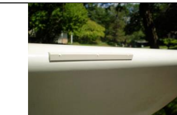
A 90-degree sharp edge stall strip is added to the leading edge of the Grumman Lynx leading edge to lower the stall angle in the root area of the wing. This alternative to washout works when inverted too.
